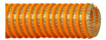
PSN is lightweight, high quality PVC hose specially designed for suction or transfer applications where visual flow is preferred. It is constructed from a very flexible corrugated, clear PVC with a smooth bore, and an external rigid orange PVC helix that allows for easy dragging. 5F to 150F.
